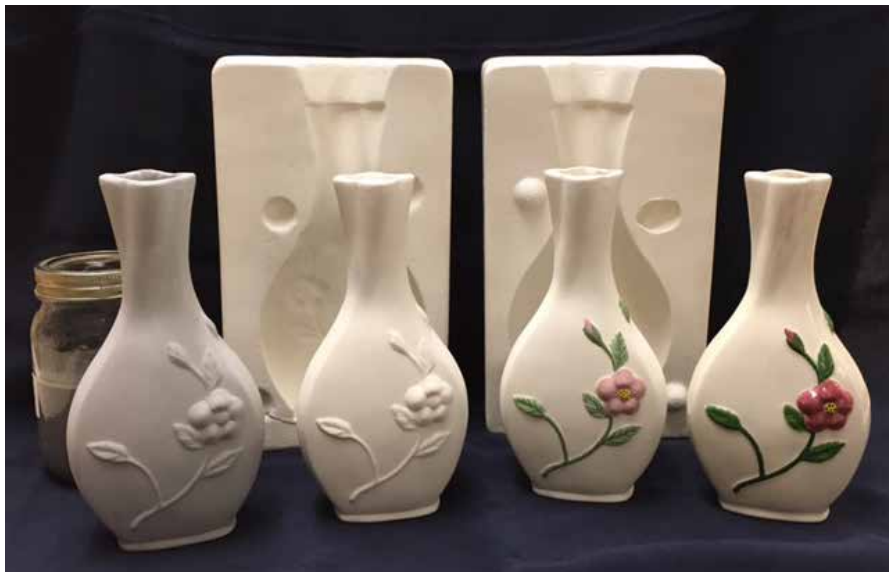
The back row shows liquid clay in jar and a two-piece mold for a vase; in the front row are, from left to right, a greenware vase, bisque vase, bisque vase painted, and bisque vase with final glaze. Vases made by Ghodsi Vakily. Photo by Gail Bragg
