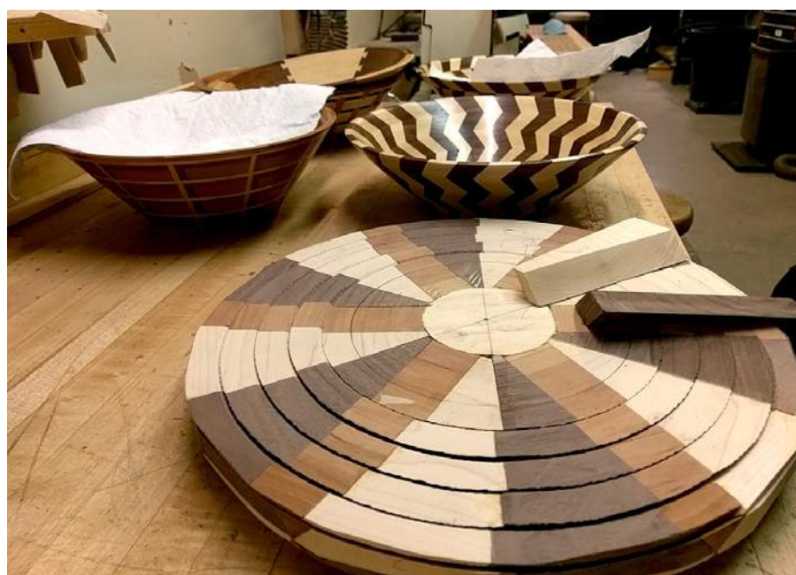
Lo's bowl-making method begins with gluing together thin chunks of wood into a disk, and then slicing the disk into rings. Photo by Kimberly Y. Choi
